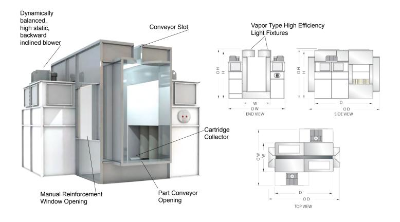
**Spray Systems** will design a customized automatic powder booth to meet your powder application requirements, specifically based upon your part size and production speed. Includes gun slots for automatic gun movers, manual operator openings, conveyor slots, conveyor openings with vestibules – all designed to meet the specific functions required by your powder production line.
