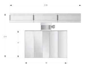
DP-1-Full Downdraft Prep Station better contains all dust particles by using a full downdraft airflow along with gravity by using a below-grade pit design. Customer should consult Spray Systems advisor before customer installs the exhaust pit
