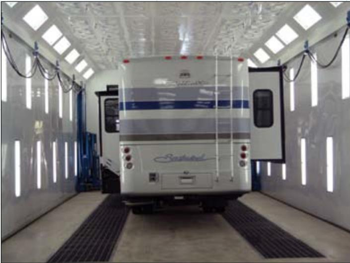
High production of large products using high efficiency down draft design
